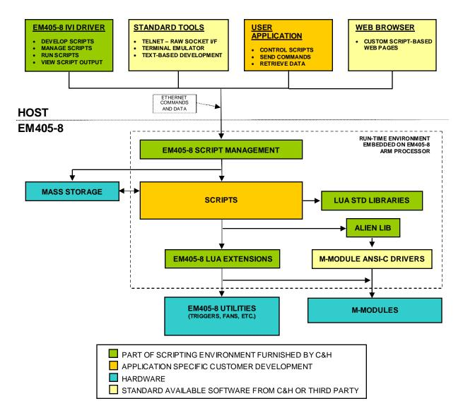
Figure 1 EM405-8 Scripting Utilities Architecture Diagram
